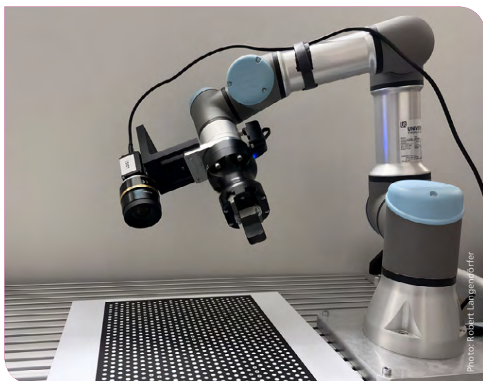
Robot calibration: Imaging a calibration body
