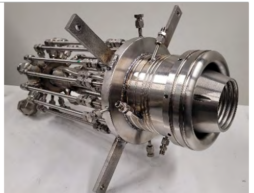
Detonation burning chamber of the third generation: With improved cooling and steam injection for coupling with a turbine. (Photos: Joachim Grune / KIT)
