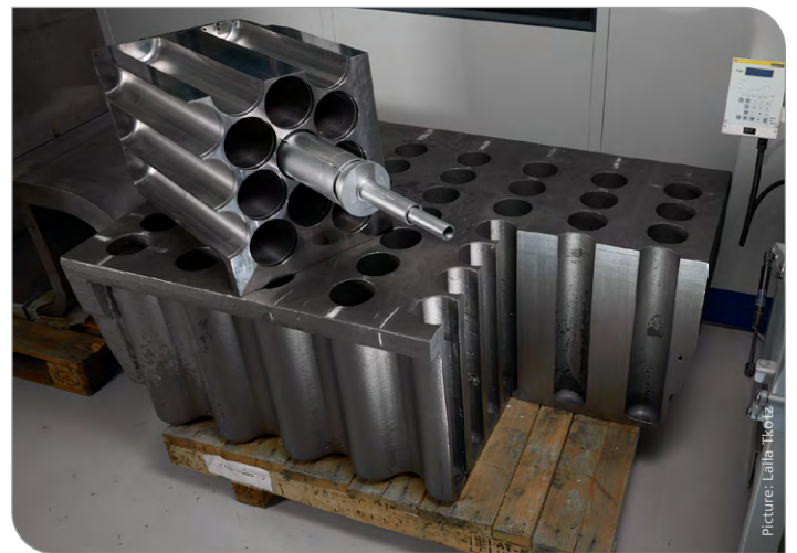
Pin monoblock prototype of the HCPB-TBB
